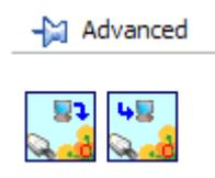
The MBVTCP\_SendRequest.vi sends a request to a ModBus server and returns a reference to this request through the *Expected answer* field. This reference is used to get the associate answer with MBVTCP\_ReceiveResponse.vi.
